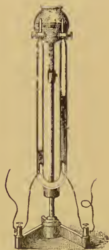
FIG. 10.—DECOMPOSITION OF WATER BY THE ELECTRIC CURRENT.
